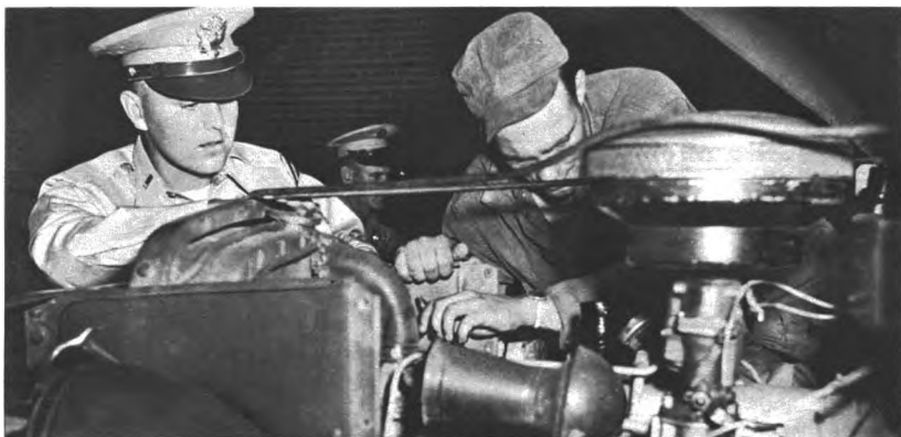
AN EXPERT'S JOB. Vanderbrugen has responsibility for care of company's motor vehicles; here he conducts routine check on truck. Preventive maintenance demands frequent inspections. Machinery and parts are replaced before break-
